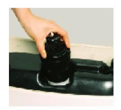
Step 9. If the tank continues to run, remove the FVC and check that the lower piston is in the proper position and check the large o-ring to ensure that it is properly seated. When the vessel is filled and the water stops running, it is an indication that the vessel is filled and ready to continue normal use.
