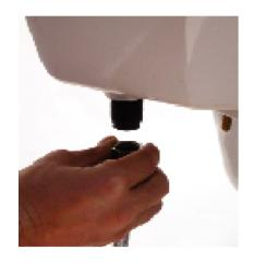
Step 2. Check for debris in the filter screen system at the water inlet for any obstruction that might limit the flow of water into the vessel. To do this shut off the water supply, flush the unit to relieve any pressure and disconnect the water supply line from the threaded connector. You can remove the filter screen easily using a set of long nose pliers. Clean and replace the filter screen, then reconnect the water supply and check the water flow
